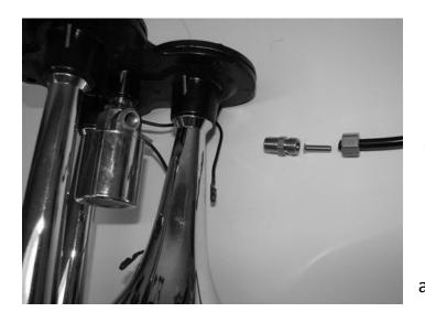
Air line to the horn solenoid: The brass 1/8" NPT Male compression fitting will need to be installed to the horn solenoid (electric valve).
