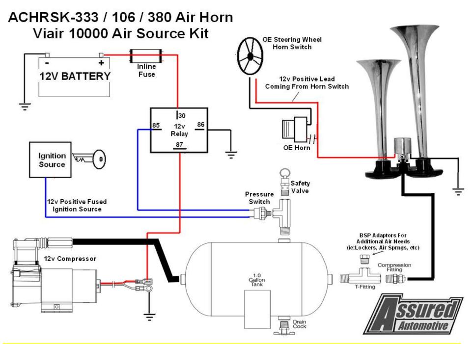
NOTE: Mount Compressor in a relatively dry location. Mount horn trumpets facing in a downward angle to prevent contaminants from sitting in diaphragms.
